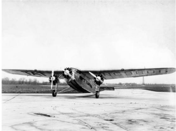
Ford TriMotor Airplane, possibly on nation's first concrete runway in Dearborn, MI
