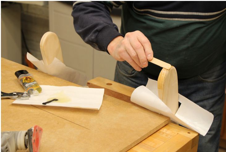
Berg Applying Epoxy to Feet
