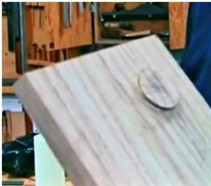
Drill tearout repair glue in
