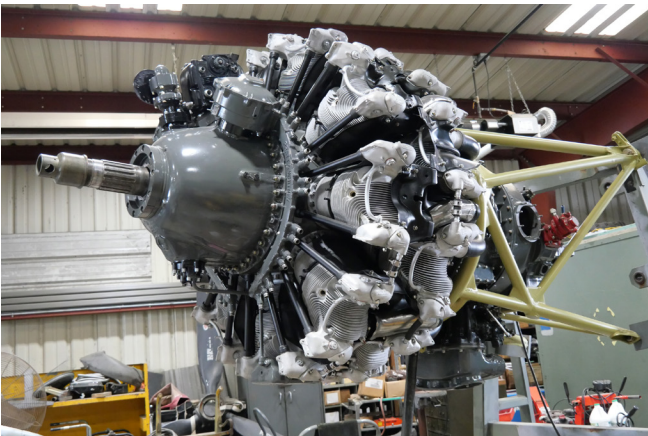
Restored Pratt & Whitney R-2800 Double Wasp Engine
