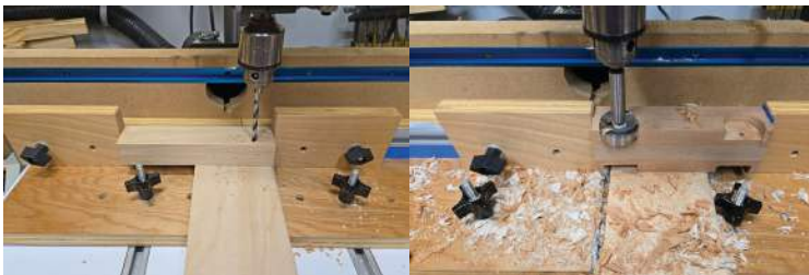
Drilling Axle Holes
