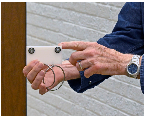
Ken's Overhead Rail Carriage
