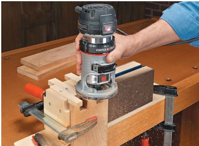
Woodsmith Finger-Joint Jig in Action
