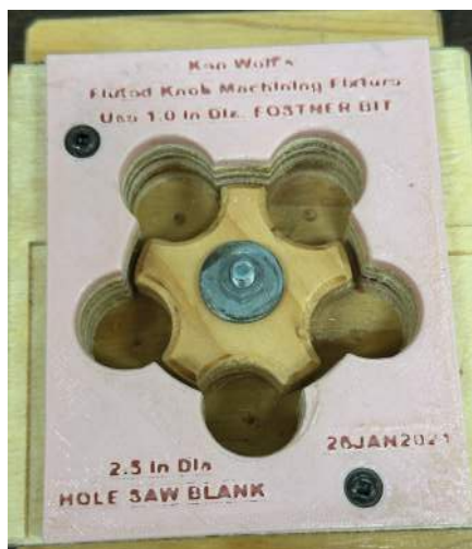
Ken Wolf Knob Machining Fixture
