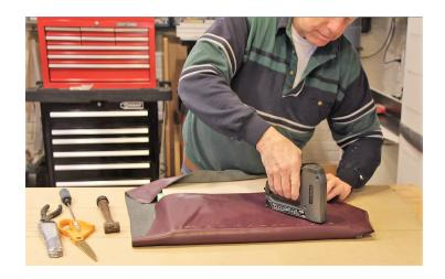
The final steps are to build the seat, attach seat support blocks to the rails, and add the strengthening corner blocks between the front legs and seat side rails. Berg makes the seat out of Baltic Birch plywood, with a leather or fabric material stapled over a foam pad.
