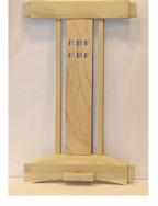
(with square cutouts near the top of slat), or a mission style chair (with the wide splat replaced with three individual slats). The splat's and any slat's top tenons for all three designs are all cut straight in line with the axis of the piece. The bot-
