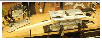
appropriate spacer wedges. And the mortises could be made with an appropriately augmented mortising machine, again using spacer wedges. But to satisfy his daughter's request to make 8-10 chairs Berg took advantage of the Leigh FMT Pro Mortise and Tenon Jig (About \$1,200 at Woodcraft) which is used with a plunge router.
