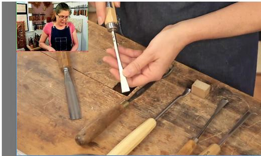
(incannel) unlike most others with the bevel down. There are also V chisels of various sizes and angles as well as gouges
