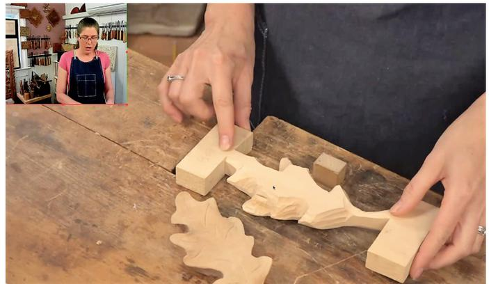
As to workspace, one can work anywhere there is tabletop with space enough for carving and tools. One must be able to secure the workpiece to table to enable control and safety. She uses bench dog clamping 90% of the time. Mary also showed a cool Sjobergs portable workstation which can be placed on any table or bench, raising the work surface about five inches. This is available locally at Performance Line Tool Center, or Glenn Wing Power Tools, or Affinity Tools Works LLC. She said cost
