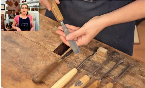
with about a 4-1/2 inch handle and a five inch straight blade curved around its axis. There are also *Fishtail* gouges, with normal width cutting edges which then taper back to a narrow shaft at the handle. Mary vastly prefers these as they are really good for getting into tight spaces.
