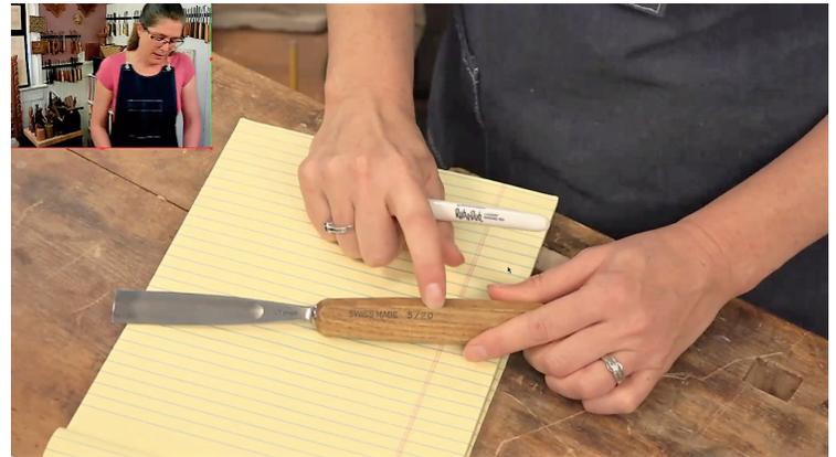
There is a two-digit numbering system for gouges, which characterizes a gouge by its cutting curve (called the "sweep"), and its cutting width in millimeters (mm). For example a #1/10 is a flat blade 10 mm wide. A #2 is slightly curved, a #3 more curved, etc. all the way up to a #11, with the aforementioned U-shape. The V tools are sometimes numbered as a No. 12 or higher.
