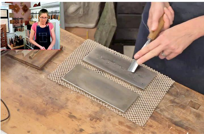
moves her body side to side, sliding the stone side to side while synchronously rotating the tool around its axis to roll the entire bevel onto the stone. If one does not roll evenly you will get flat spots. And the wedge side of the bevel should be perfectly flat axi-
