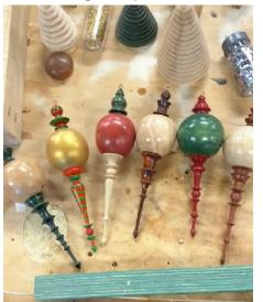
tion of the Mike Foydel shop tour showing a demo of making Christmas ornaments, one with a round hollow ball with long thin finials on the top and bottom, and another in the shape of a snowman. The ball starts with a cylinder which is hollowed out and
