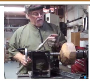
his gouge very sharp, Mike's shavings were very long and uniform. He reminded us to occasionally tighten the headstock on the damp tenon since the wet wood can shrink or compress as it dries out.
