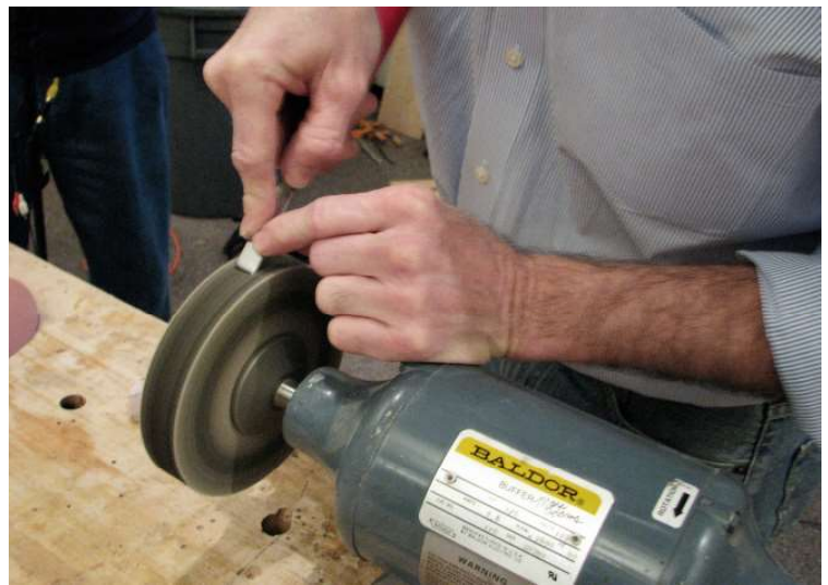
Marc is buffing the chisel to remove the burr. Note that the buffer is rotating away from him
