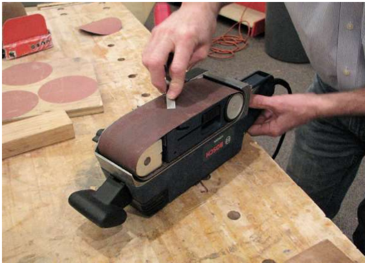
Marc Adams demonstrating how to sharpen a chisel on an inverted belt sander
