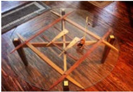
The glass was made to float above the leg assembly with wood pegs, and some decorative triangles of figured wood were added under the glass. And he showed a smaller long hall table, rectangular with floating glass. Under the glass was a long figured piece with a pair of little Koa wood tabs (like an equal sign “=”) as accent pieces. Koa wood comes from Hawaii. Will has made about 10 copies of this popular convenient size table, all with different woods and accents.
