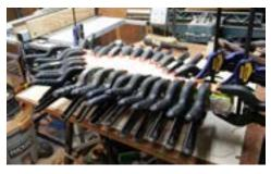
2 pine cut with a 15° angle. These strips were then glued together with canvas sandwiched in-between. (To make the glue-
